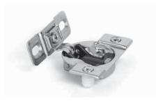
**COMPACT BLUMOTION 38B face mount hinges for full overlay** Full overlay face mount hinges with a 107° opening angle and 7/16" cup depth
